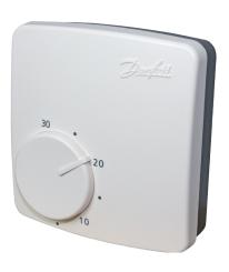
The RET230P electronic room thermostat is designed for accurate control of central heating systems. Using a 230Vac mains supply, the voltage free contacts can be used for either mains or low voltage switching systems.
